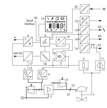
Fig. 5: Functional diagram of Type 3730-2 Positioner
